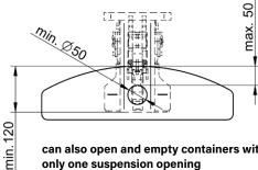
can also open and empty containers with only one suspension opening
