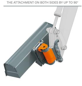
WITH THE TC TILT COUPLER, PRECISE ANGLE LEVELLING OF EMBANKMENTS IS NO PROBLEM
