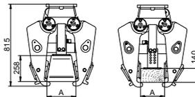
Internal pads and adjustable plunge depth allow the gripping of MonoBloc sleepers of different sizes and material (concrete, wood)
